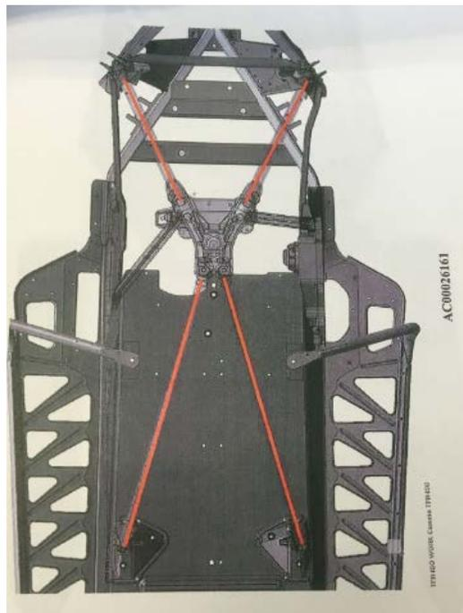
(First Farco Decl., Ex. H at H-9 (photos of the F4 Chassis).) Arctic Cat has referred to the brace assembly of the F4 Chassis as a “pyramid design,” just as it did the Sno Pro Racing Chassis. (See Farco Decl., Ex. C at AC.RF.012560 (“The pyramid designs of these race-proven chassis . . .”).)
